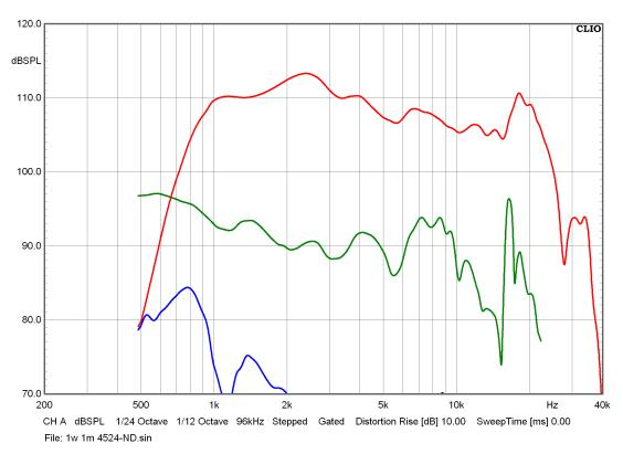
4526ND-8 in 90° x75° CD horn, 2nd and 3rd harmonic distortion raised 10 dB, SPL 1W/1m
